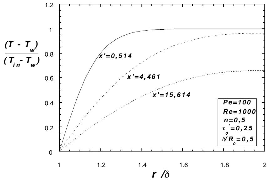
Figure 7: Dimensionless temperature profile for different axial positions,  $T_w = \text{constant}$ .
