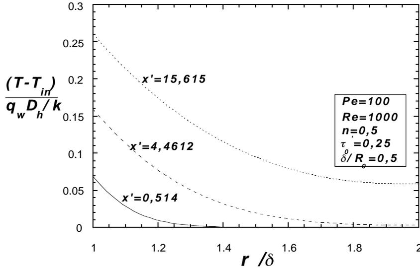
Figure 2: Dimensionless temperature profile for different axial positions,  $q_w = \text{constant}$ .
